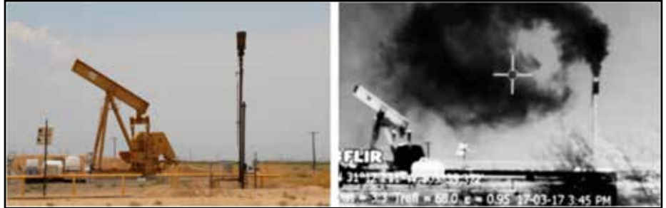
Left: a normal view of Reeves County oil and gas facilities. Right: infrared view of the same facility, showing normally invisible pollution.
