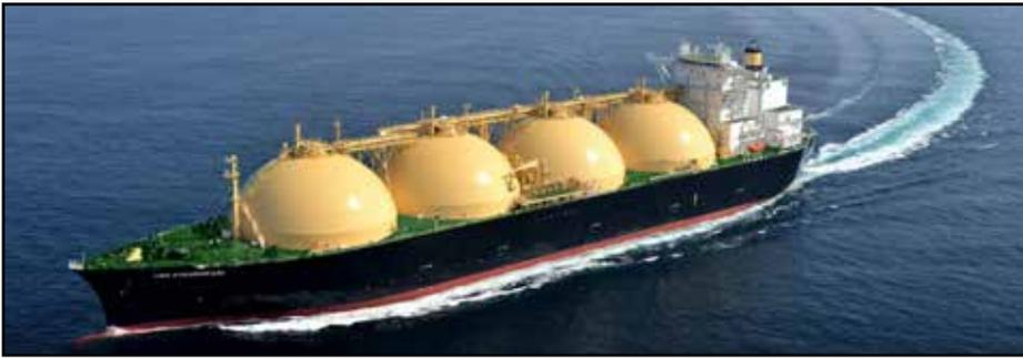
LNG ships like this one will sail into Eastern Australian terminals and discharge gas at  $-161^{\circ}\text{C}$  – usually to another vessel, a floating storage and regasification unit (FRSU). Seawater is used to warm and regasify the liquid. Photo: APLNG
