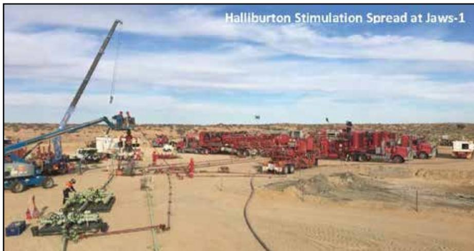
*Halliburton contractors fracking Strike's Jaws-1 CSG well using an extreme new technique. Photo: Strike Energy*
